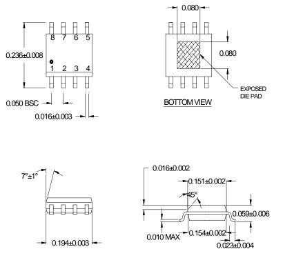
3. UNIT = INCH MOLD FLASH, PROTRUSIONS AND GATE BURRS AT THE END OF THE PACKAGE BODY SHALL NOT EXCEED 0.006" PER SIDE.
